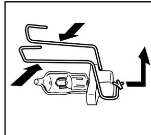
3. Tip the grille forward, then lift out to remove.
